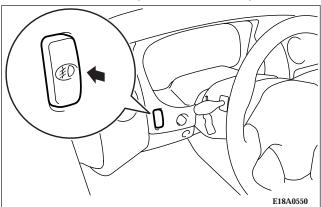
The fog lights illuminate only when the headlights are on. Press the switch to illuminate the fog lights and press the switch again to turn the lights off.
